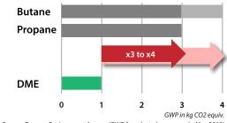
When a propellant is used, it is released into the atmosphere. Consequently, the global warming potential becomes relevant.
